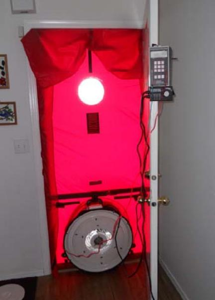
Done with a blower door tests with air handler on and off
